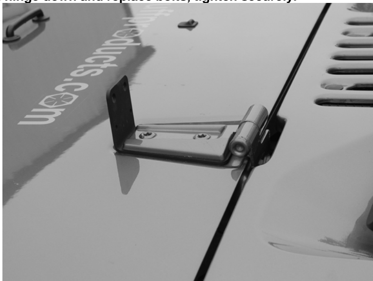
Step 5: Fold hinge down and replace bolts, tighten securely.
