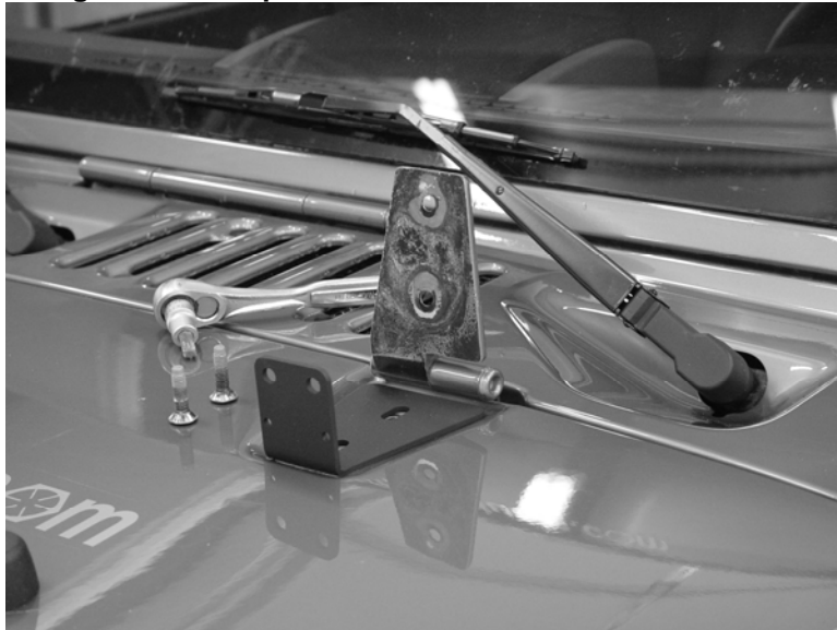
Step 5: Fold hinge down and replace bolts, tighten securely.
