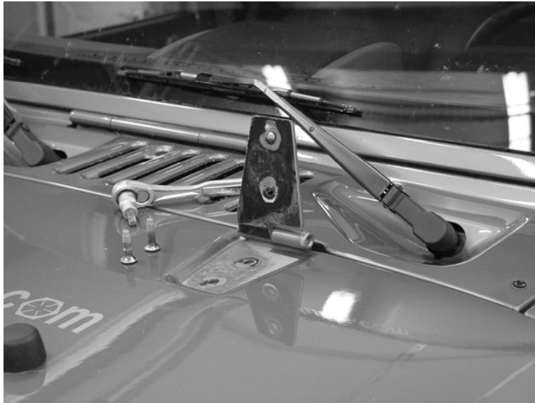
Step 4: Place Hinge Bracket in place.
