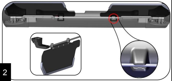
Next, install the left and right Axis Sun Visor Mounts, using the screws that were removed from the factory sun visors in step 1. **Note:** If holes do not line up, then loosen the right side rod mount bolt (1/8" hex bit) and adjust position of rod and mounts as needed. Once mounts are installed retighten rod mount bolt.
