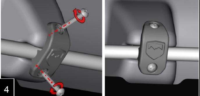
**Note:** The Axis Sun Visor has 2 friction setting bolts and 4 mounting bolts. The upper 4 mounting bolts (pictured) should be kept tight and not be loosened to adjust rotational stiffness. The lower two bolts can be tightened or loosened to adjusted for rotational stiffness.
