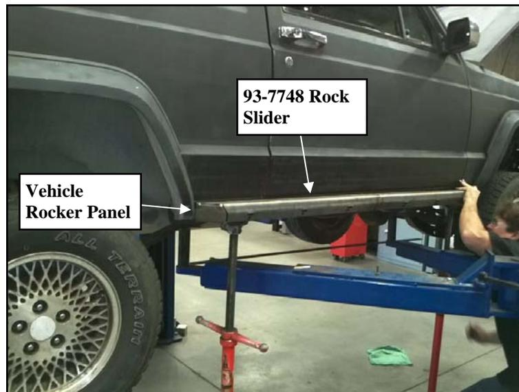
**Step 3:** Once confident with the slider location on the vehicle, center punch the (**6 per side**) side mounting hole locations and (**4 per side**) lower mounting hole locations using the supplied transfer punch (**90-4432**). (Fig. B)
