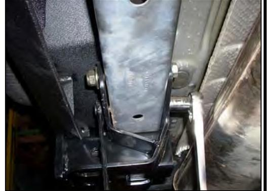
4. Insert the trailer wiring, if equipped, into the trailer wiring mounting tab on the receiver as shown. Installation is now complete.
