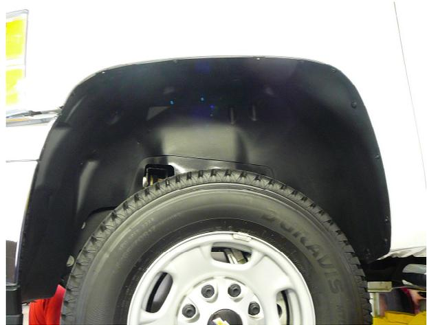
**STEP 4:** Clean the body areas where the Fender Flares will make contact. Ensure fenders are dry prior to install.
