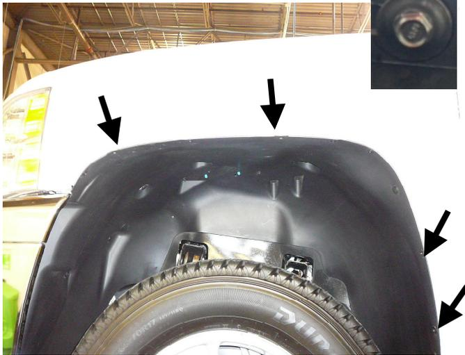
**STEP 5:** Place the Fender Flare on the vehicle into the position of best fit. Note where the slots in Fender Flare at positions **A, B, C, and D** align with the existing screws in the vehicle. Remove Fender Flare. Use the original manufacturer's hardware that is in the wheel arch of the vehicle to fit the Fender flares. Remove the x4 9/32" (7mm) socket head screws from the fasteners on the vehicle.
