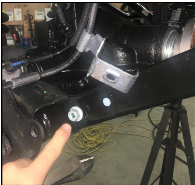
Remove Brake Lines from Arms
