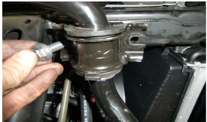
Install the ReadyLIFT sway bar brackets to the frame with the offset holes forward. Use **factory hardware**. Torque to **35 ft-lbs**.
