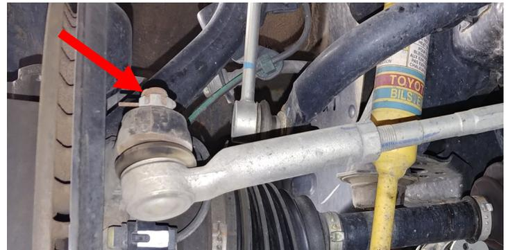
Remove the sway bar from the frame rail. Let hang out of the way.
