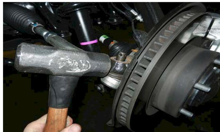
Remove the **lower strut hardware**. Retain lower hardware.
