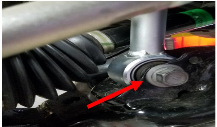
Loosen but do not remove the **upper control arm hardware** to allow the bushings to relax and have the suspension droop out. Make sure the CV axles do not over extend.
