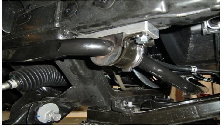
Install the wheels and lower the vehicle to the ground. Torque the lug nuts to the wheel manufacturer's specs. Jounce the suspension to get it to settle to the new ride height.
