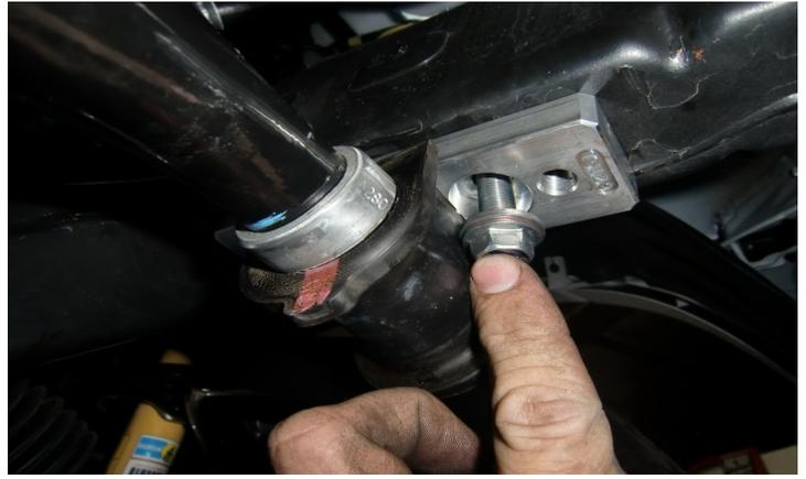
Install the sway bar to the ReadyLIFT brackets using the **provided hardware**. Torque to **35 ft-lbs**.
