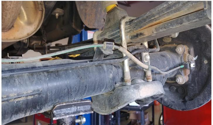
Lower the axle low enough to install the ReadyLIFT block. If the block is tapered, make sure the small end of the block is towards the front of the vehicle. Raise the axle while lining up the center pins. Install the provided u-bolts and hardware. Do not tighten fully, leave loose so that you can repeat the steps for the opposite side. Repeat all steps above regarding the block install.
