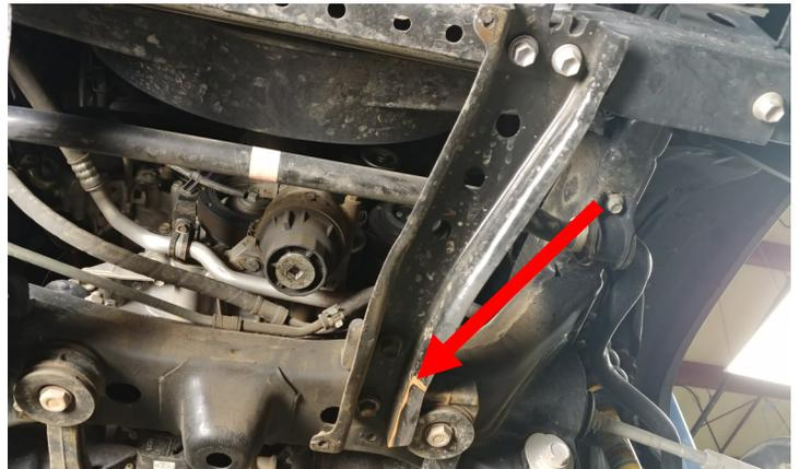
If so, **mark the protruding area** with a suitable marking tool. Remove from the vehicle and use a suitable cutting tool to trim off the marked section. Sand off any burs left over from the cutting. Use a quality rust-preventative paint on the exposed metal.
