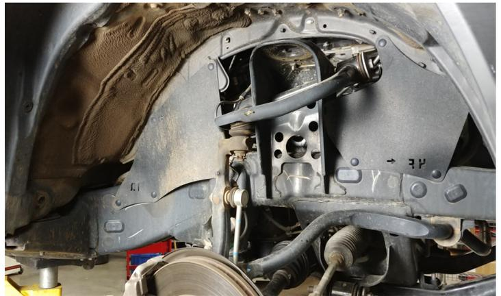
Install the new **strut assembly**. Use the **provided hardware** to secure the strut to the strut tower. Leave the nuts loose, you will properly torque these when the vehicle is lowered to the ground.
