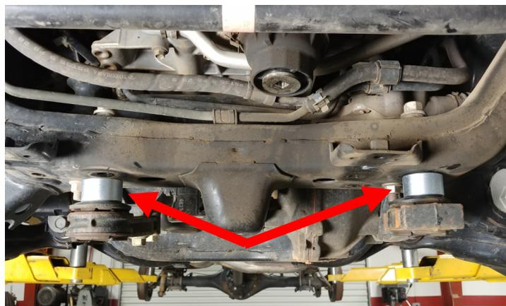
Attach differential brackets with provided hardware. Use factory large bushing washers in their original location. Torque to **95 ft-lbs.**
