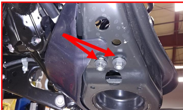
Loosen but do not remove the lower control arm cam bolt at the subframe.
