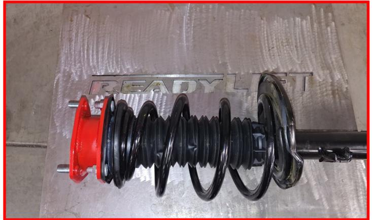
Install the completed strut assemblies back into the vehicle using the factory hardware. Only start the nuts by hand to allow movement when installing the knuckle. Make sure to install the hardware in the same locations as previously removed (**outer nut circled in red**).
