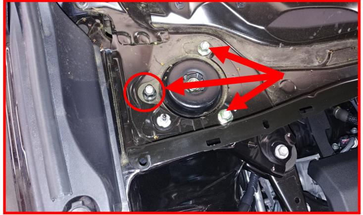
Install the ReadyLIFT strut extensions to the strut top hat using the provided **M10 flange nuts**. Torque to **30 ft-lbs**.
