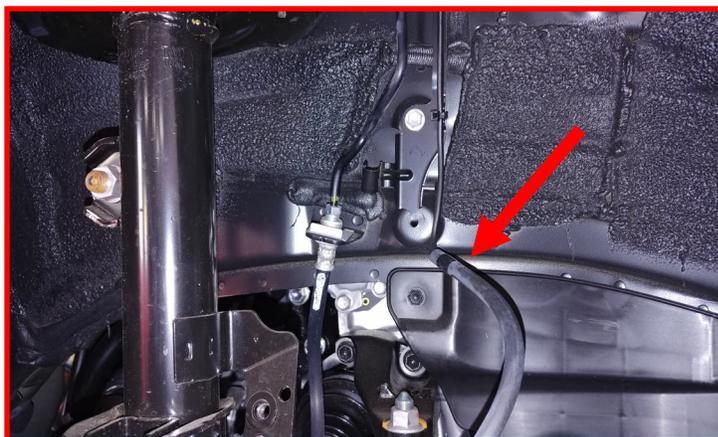
Remove the sway bar end link from the strut body. Let hang out of the way.
