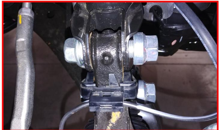
Install the ReadyLIFT sway bar bracket to the strut body using the provided **M12 bolt, washers, and nuts**. Install the sway bar end link to the bracket using the **factory hardware**. Torque all to **45 ft-lbs**.
