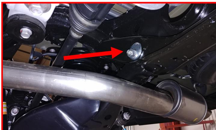
Loosen but do not remove the front lower control arm mount.
