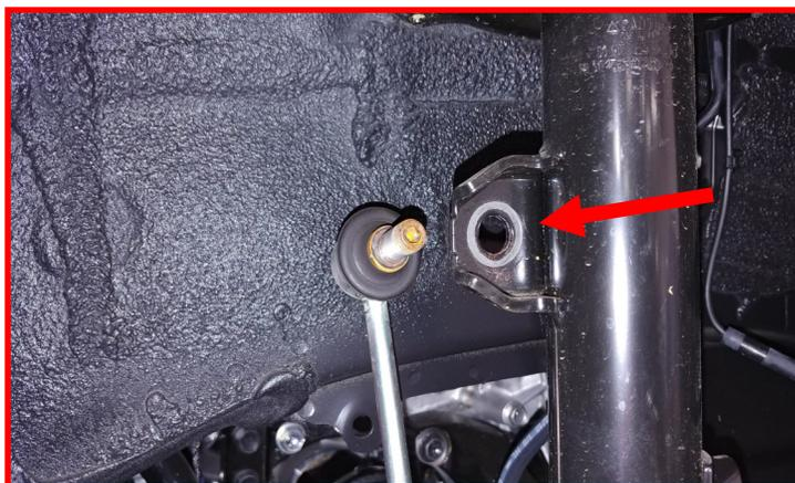
Remove the two bolts holding the strut to the knuckle.
