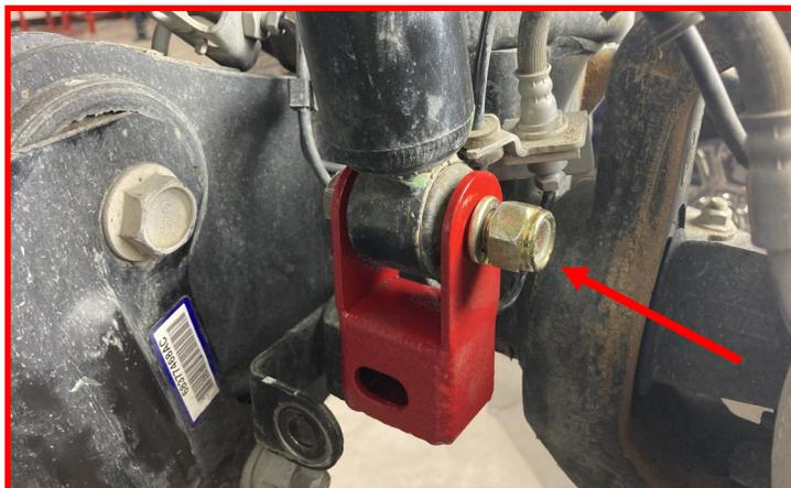
Install the lower bolt of the **shock extension** using the **factory 21mm bolt**.
