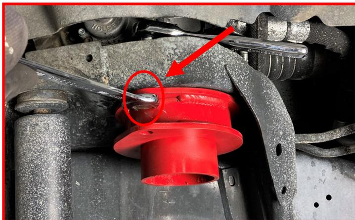
Place the spring isolator into the bottom locating hole on the **spring spacer**.
