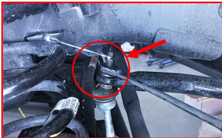
Remove the 21mm lower shock bolt.
