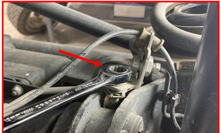
Loosen and then re-tighten the track bar bolts at the frame and axle ends.
