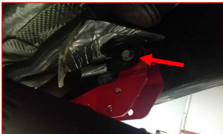
Install the ReadyLIFT control arm bracket to the lower control arm pocket using the **factory hardware**. Do not tighten at this time.
