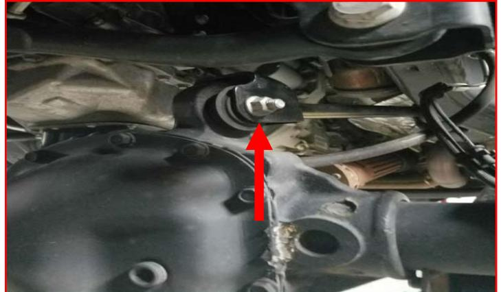
Loosen but do not remove the lower control arm bolt at the axle.
