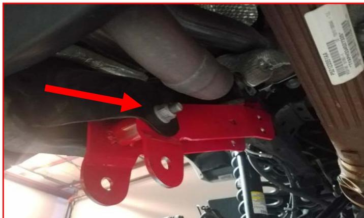
Install the upper arm to the bracket (use the upper hole for 2.5" lift heights, and lower hole for 3-4" lift heights) using the provided M12 x 80 mm bolts, washers, and nuts. Install the lower control arm to the bracket using the provided M14 x 100 mm bolts, washers and nuts. Do not tighten at this time.
