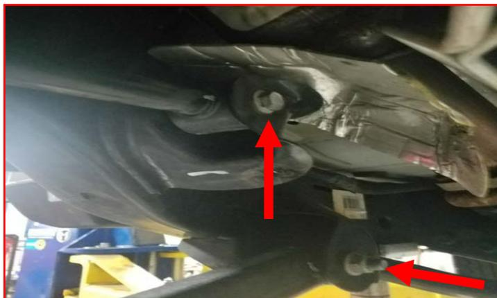
Install the ReadyLIFT control arm brackets to the upper control arm pocket using the **factory hardware**. Driver and Passenger sides marked with D and P respectively. Do not tighten at this time.
