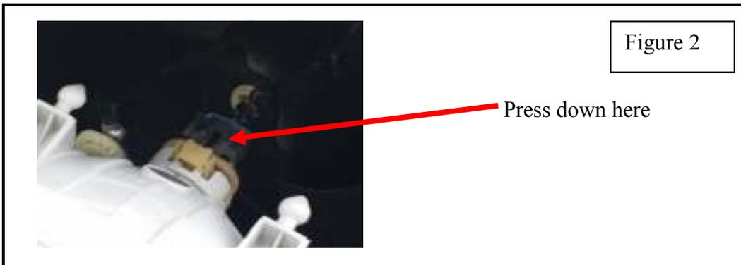
3. Remove fog lamp assembly and set aside for next step as some parts are reused.
