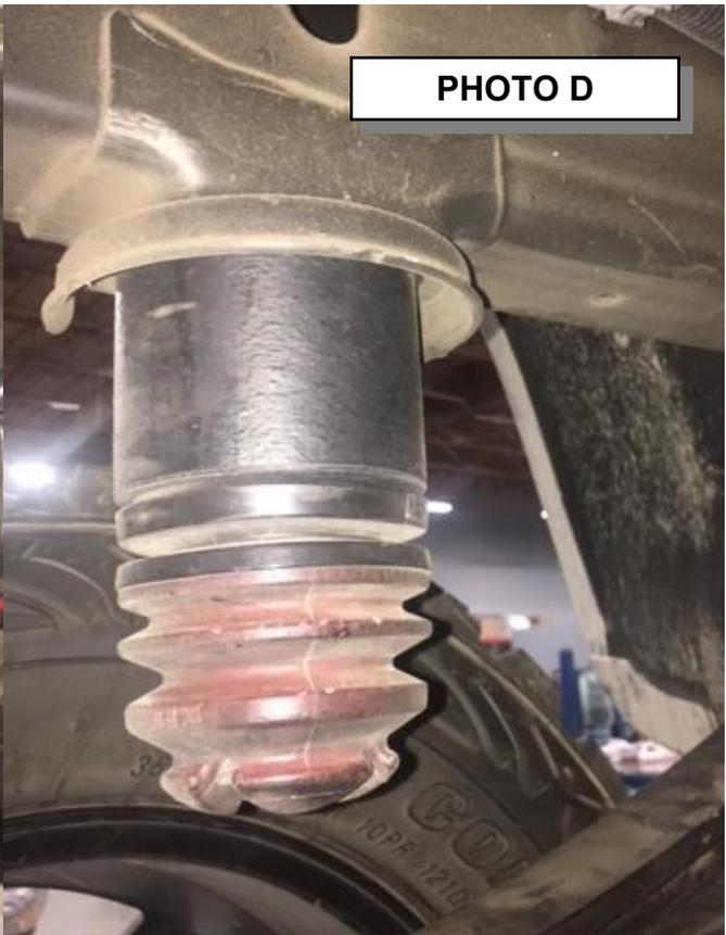
the shock mounts. Carefully check for clearance issues. If there are areas that come in contact with or are very close to your new shocks, carefully remove sufficient material to ensure trouble free operation. Pay particular attention to the area around the lower shock mount. When all clearance issues have been resolved, install your new Pro Comp shock absorbers. Torque the upper bolt to 70 ft./lbs. and the bottom bolt to 118 ft./lbs. Re-check all fasteners for proper installation and torque.
