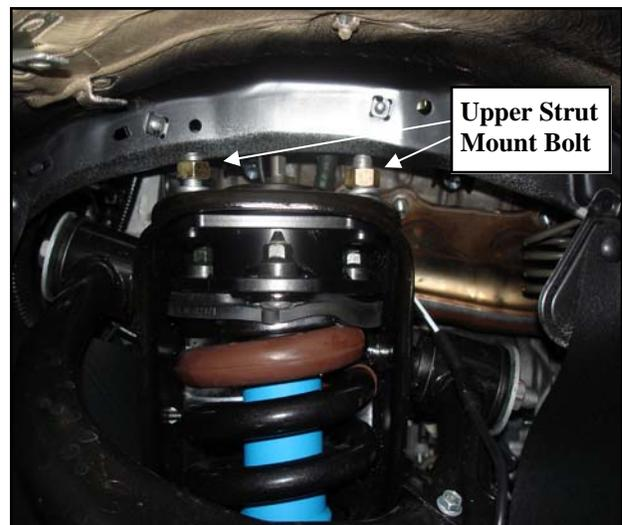
9. Remove the strut assembly from the vehicle and install securely in a bench vise.
