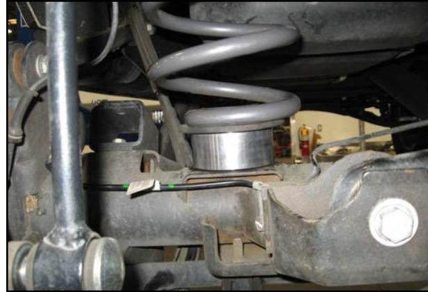
14. Reinstall the lower shock mounts using the previously removed OE lower bolts. Torque per OE specifications.
