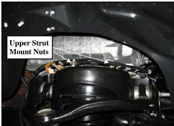
14. Carefully remove the strut assembly from the vehicle.
