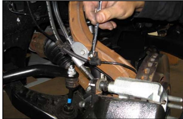
9. Unbolt the upper ball joint nut, but **DO NOT** remove it from the knuckle. Separate using the appropriate tool.
