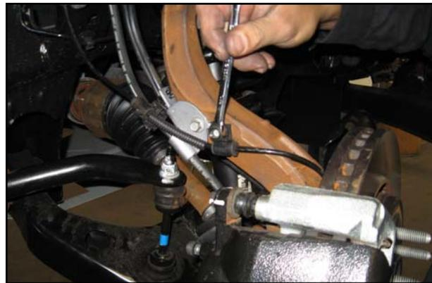
9. Remove the vacuum line from the back of the hub.
