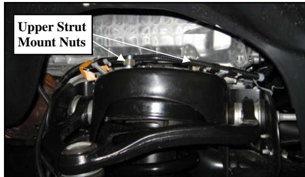
19. Remove the strut assembly from the vehicle.
