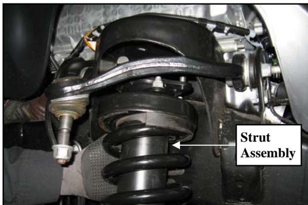
15. Install the strut spacer (94-2834m) onto the OE strut mounting studs. Secure with the previously removed OE nuts. Torque the nuts to factory specifications.
