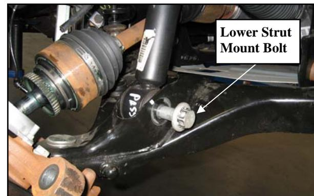
11. Support the lower control arm with a floor
