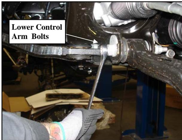
12. Push down on the lower control arm in order to dislodge the strut from the lower mount.
