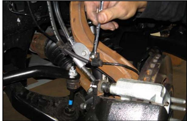
9. Remove the vacuum line from the back of the hub.
