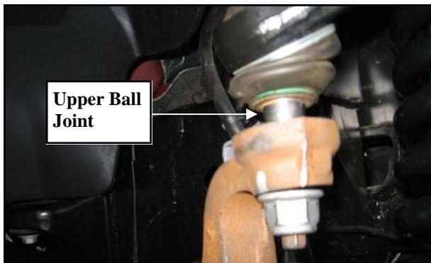
15. Remove upper ball joint nut and carefully lower the A-arm assembly. Save hardware for reinstallation.
