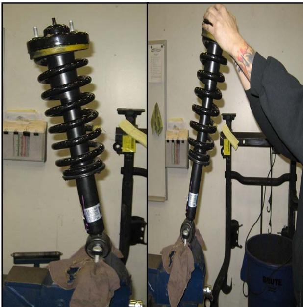
24. Install the strut assembly into the strut tower and start the (3) upper 10mm flange nuts. (Make sure that the bottom of the strut is aligned as well) Torque the upper strut tower 10mm nuts to 60 ft./lbs.
