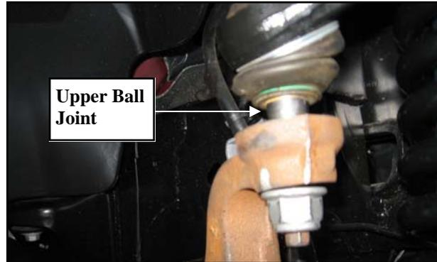
9. Remove upper ball joint nut and carefully lower the A-arm assembly. Save hardware for reinstallation.
