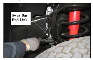
7. Support the front axle with a jack. Disconnect track bar at the axle mount and
