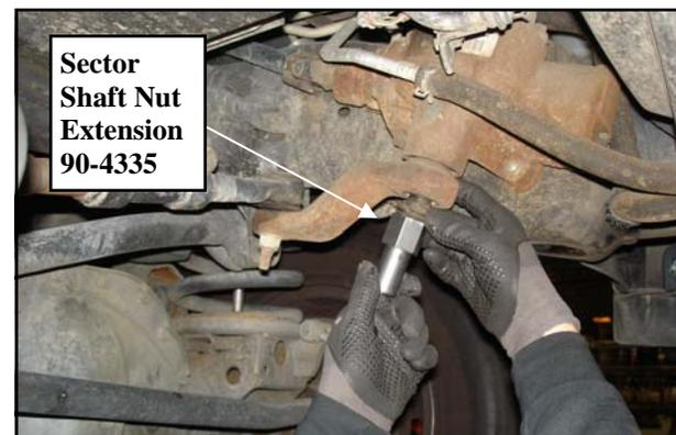
7. Torque the newly installed sector shaft nut extension (90-4335) to 180 ft./lbs. Be sure to use thread locker on the nut.
