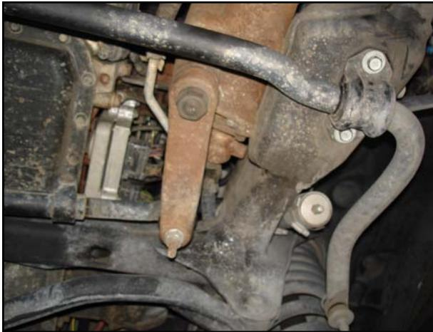
3. Carefully, unbolt the sway bar mounts from the frame. Be sure to support the sway bar so it doesn't swing down.
