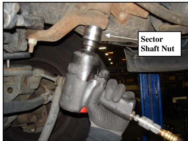
6. Install the supplied sector shaft nut extension (90-4335) and the previously removed OE lock washer.
