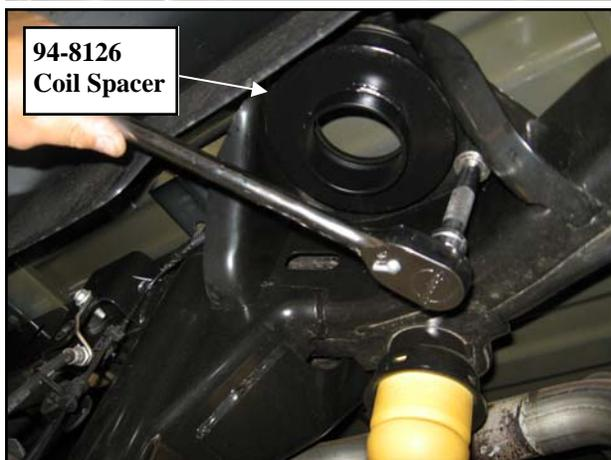
7. Reinstall the rear spring assembly into the rear axle spring perch. Make sure the pig-tail of the spring is properly indexed in the mounting pocket.
