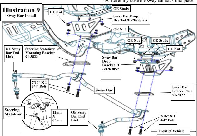
and on the passenger side insert the steering stabilizer bracket (91-3823) under the passenger side sway bar mount. On the driver side insert the sway bar spacer plate (91-3822) under the driver side sway bar mount. Secure the supplied 7/16" X 1 3/4" bolts and hardware. See ILLUSTRATION 9.
