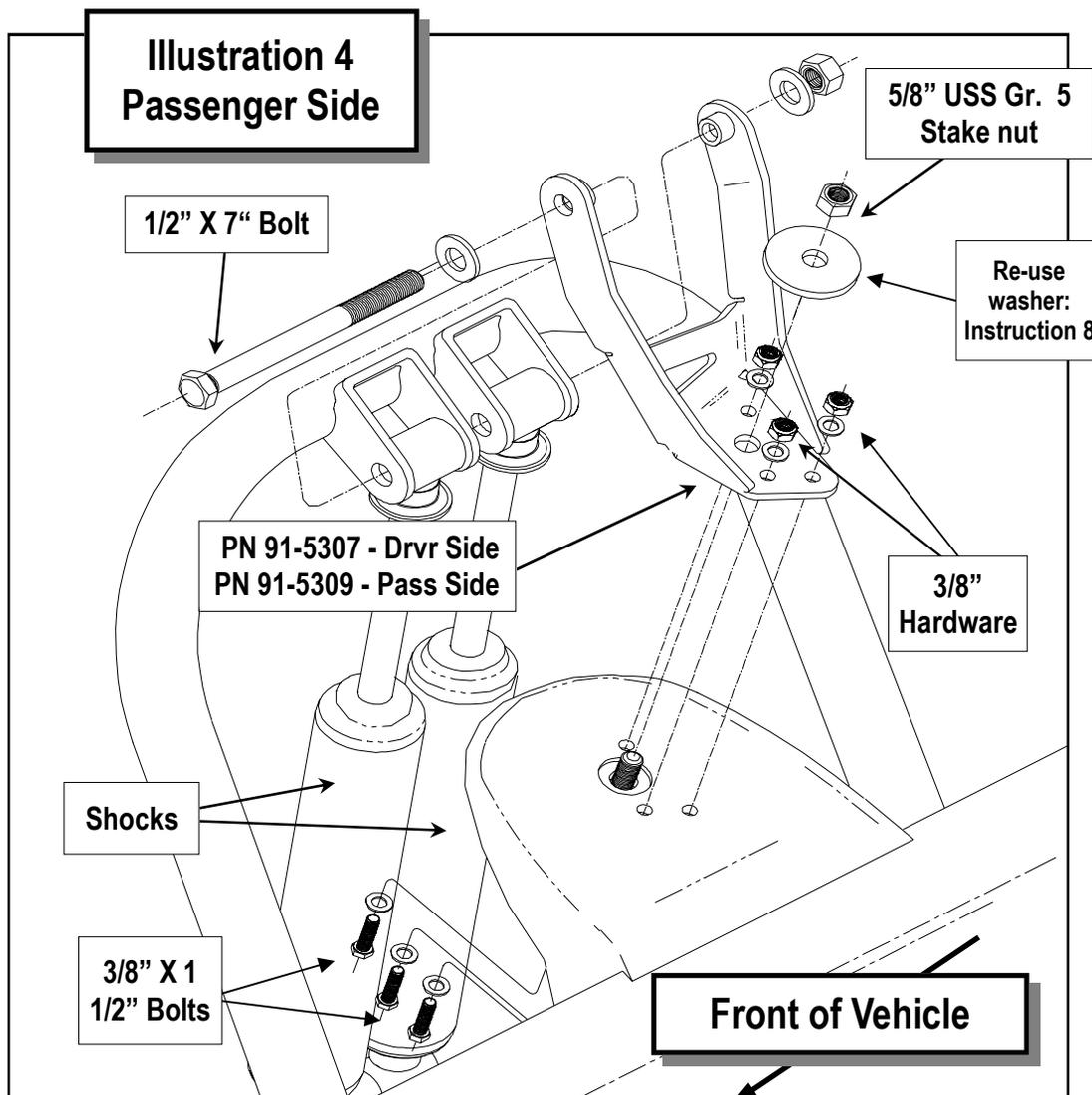
12. At this point, check the entire assembly for clearance. It is ***critical*** that brake lines and ABS wiring is secured in such a manner that there is no rubbing or scraping of these components,
