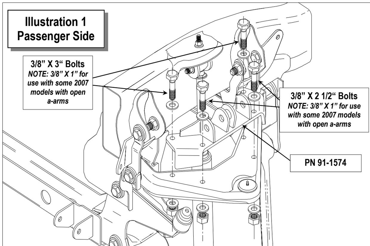
2. Remove the four **9/16"** bolts that hold the upper A-arm drops to the OEM A-arm mounts. Discard this hardware.
