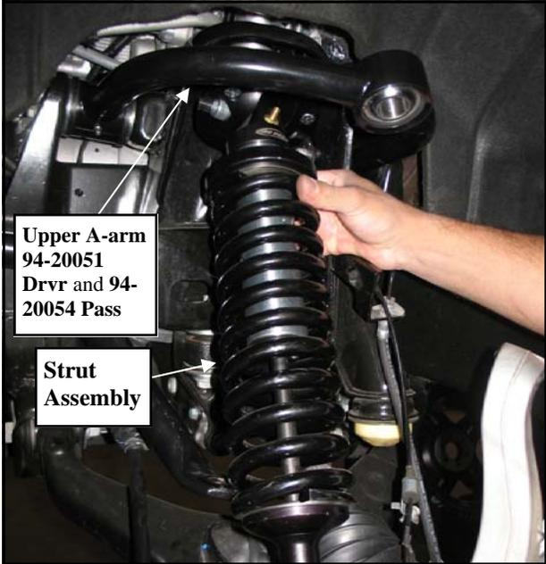
17. Install the Pro Comp upper A-arm (94-20051 Drvr and 94-20054) into the original mounting location using the previously removed OE pivot bolts, load washers (90-9607) and OE hardware. Torque according to manufacturer's specifications. Be sure to grease the bushings and load washers.
