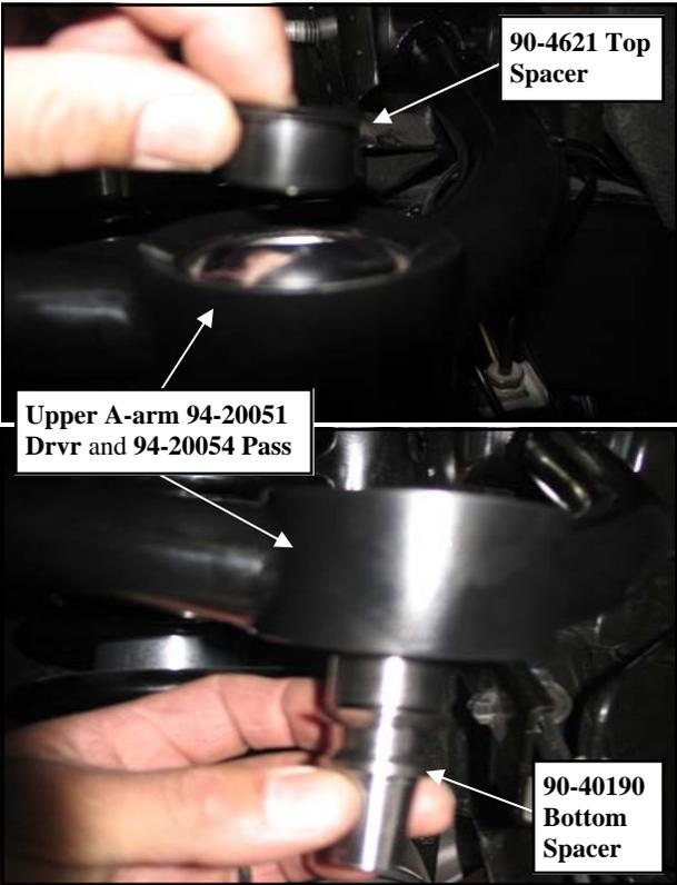
19. Raise the lower A-arm and knuckle and secure the upper ball joint mount to the knuckle using the supplied 1/2" X 4" and hardware. Torque 1/2" hardware to 80 ft./lbs.
