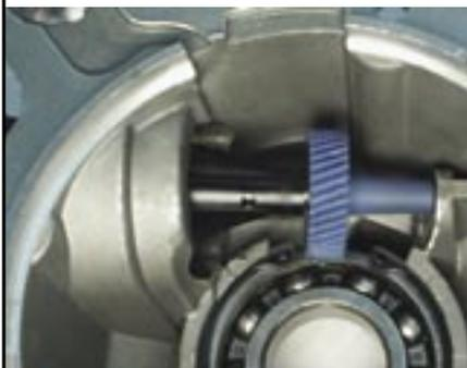
When installing the rear bearing snap ring be sure to place it in a position that will not allow the speedometer driven gear to contact the snap ring. Use this photo as a reference.
