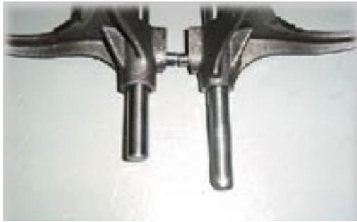
**Note:** Verify the length of your mode fork shift rod as shown. If your shift rod measures 10.2", it will need to be cut down to a length of 9.380". This is typical of 1988 and 1989 model YJ's.
