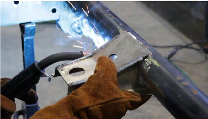
Tack weld bracket into place and test fit body bushing and bolt to check fitment.
