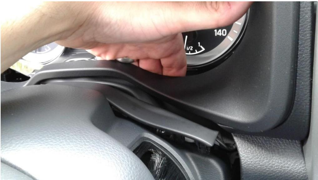
9. With access to the I/C achieved, remove the 3 phillips head screws. The cluster has small tabs that clip it in place, gently pull forward and it will come free.
