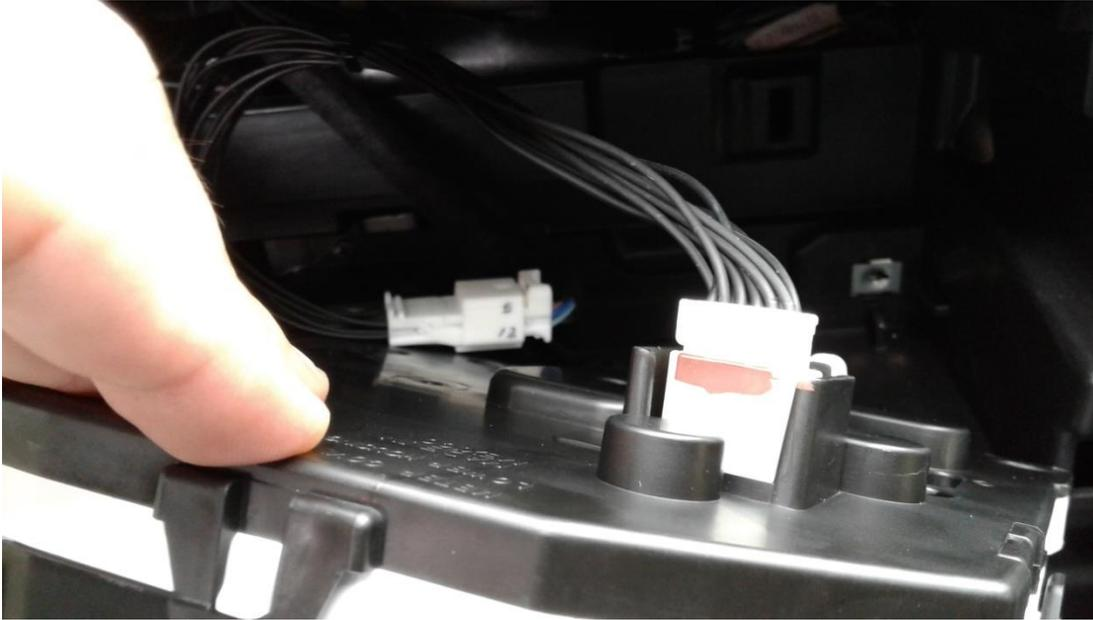
10c. Rest the module behind the main wiring harness for room and reinstall the I/C.
