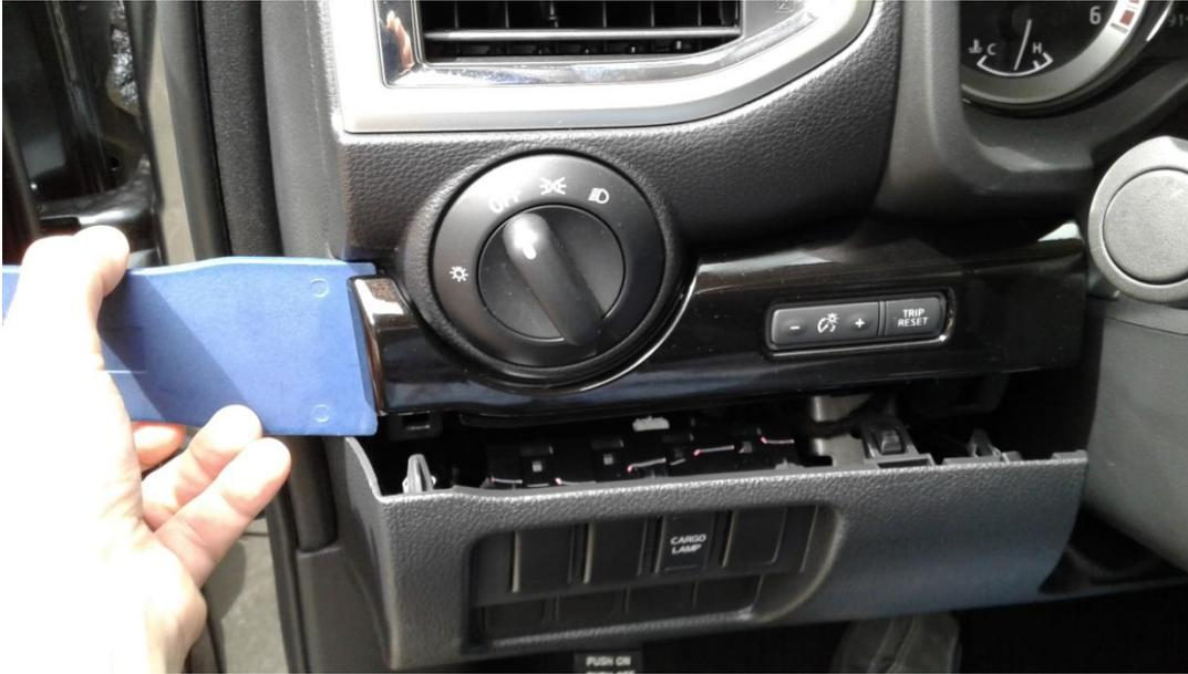
5. Insert the trim tool behind the upper I/P shroud and pull backwards to release the shroud.
