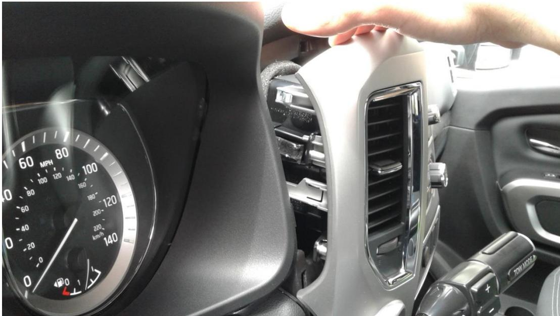
3. Insert a trim panel tool in the space between the lower kick panel and the bezel that contains the Trip Reset and I/P Illumination controls. While reaching in with your fingers on the back side, push up on the tool and pull backwards with your fingers to release the panel.
