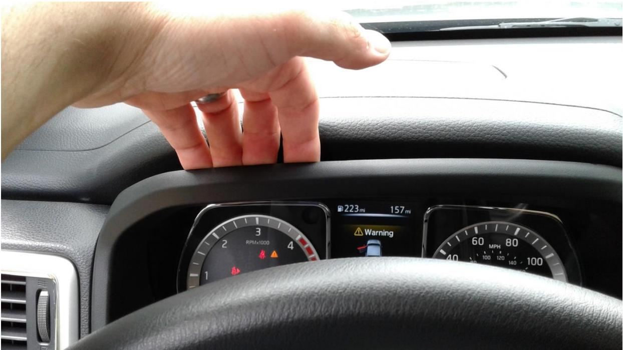
8. To remove the I/P shroud, you will need to disengage the vinyl steering column cover. Insert a small screwdriver on the left side and gently pry up to release the first clip.
