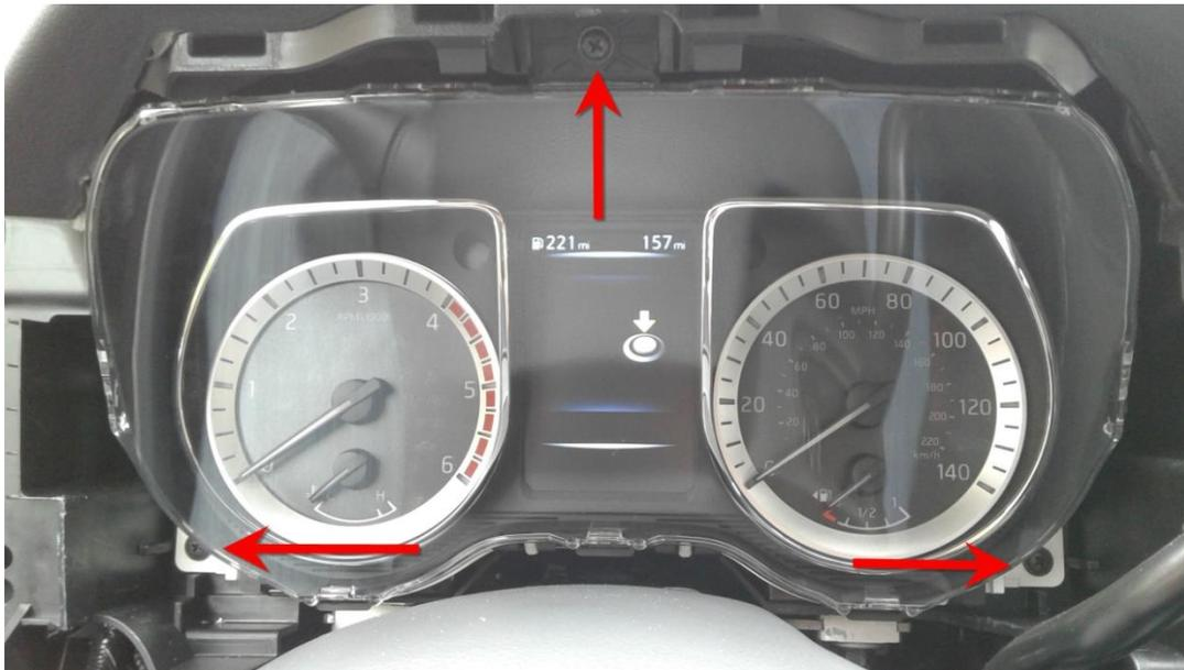
10. Pull the I/C forward to gain access to the connector and depress the tab on top and pull back to disconnect.
