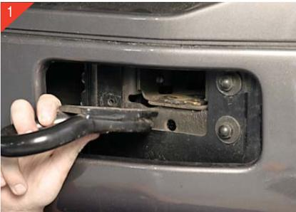
1 Start with removing the tow hooks by removing the 3 - 15mm bolts on both driver & passenger side of vehicle.
