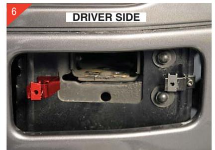
6 Next remove the brackets from the billet grille. Then attach the brackets to the vehicle in the just drilled locations using the supplied hardware. Use #8 x 1" bolts for the holes to the inside of vehicle (bracket in Red) . Use #8 x 3/4" for the outside.
