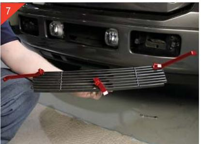
7 Next loosely attach brackets to the center section of billet grille as shown. Rotate brackets as necessary in order to place billet grille into opening and center. Then rotate the brackets out similar to the picture above and tighten so they will stay in place for marking. The long brackets will end up attaching in the tow hooks section. Then mark locations of the holes in brackets and remove grille. Then drill a 9/32" hole in each of the marked locations.
