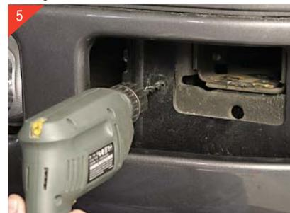
5 Next drill a 9/32" hole in each of the marked locations. It may be necessary to start with a smaller drill bit such as a 5/32".
