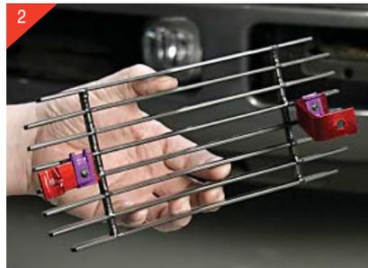
2 Next you will be attaching the brackets to the backside of billet grille as shown above. Start by attaching the supplied U-clips to each of the brackets, then attach bracket to billet grille using the supplied #8 x 5/8". Take note of the bend angle of billet grille the longer "L" bracket attaches to the long side of the grille and the bracket to the short side.
