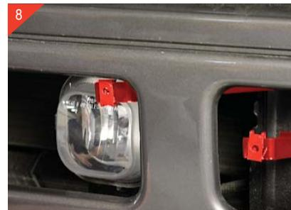
8 Next attach the brackets to the vehicle using supplied hardware #8 x 3/4". With all brackets attached to vehicle simply attach billet grilles to vehicle using supplied Phil Pan Head Screws.
