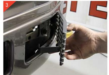
3 Place billet grille into opening and center. Take note that the shorter angle of the billet grille goes to the outside of the vehicle.
