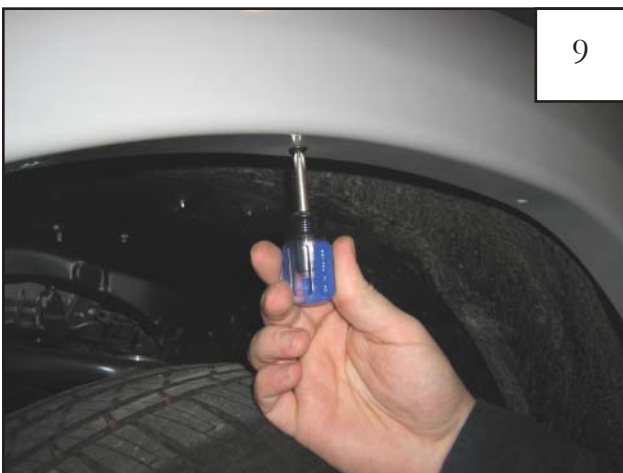
Replace flare on fender, aligning holes in clips. Start three supplied Serrated-Flange Screws through three holes in flare and into "S" Clips installed in Step 7.
