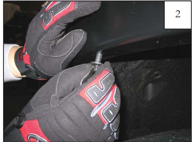
Holding flare in position on fender, install two supplied Plastic Push Retainers.
