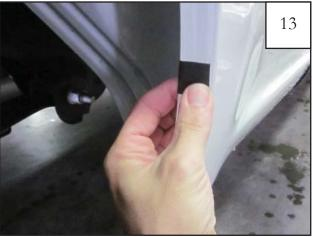
Wrap a Foam Tab (MT1-0034) around the wheel well sheet metal, centered over each of the upper four marks made in Step 12. Place a Mylar Tab (MT1-0014) at the mark made on the lower front of the wheel well.
