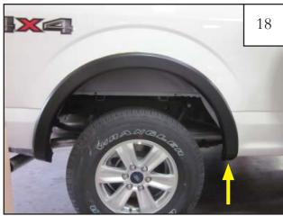
Start a supplied screw (SW1-0050) through the flare into the clip installed in Step16. Tighten all screws.
