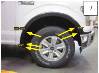
Still holding flare to fender, re-install remaining factory screws removed in Step 1 using 7/32" and 9/32" sockets and wrench. Install supplied screw (SW1-0058) into Clip (CL1-0009). Tighten all screws.
