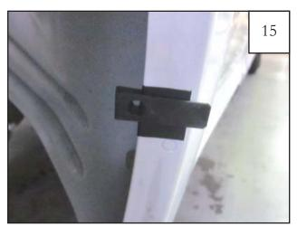
Install a Clip (CL1-0009) over each of the four Tabs (MT1-0034) placed over the upper 4 marks made in Step 13.
