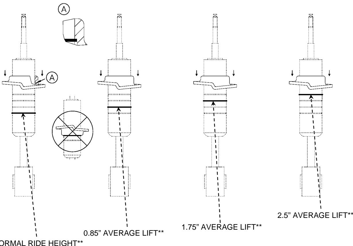
\*\* Ride heights indicated are typical. Actual ride height is influenced by which factory suspension the vehicle is equipped with and its condition; optional equipment and accessories on your vehicle, and other vehicle modifications such as replacement coil springs, wheel and tire combinations, etc.
