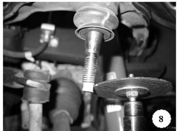
ball joints and loosely thread the nuts in place. **It is helpful to use a jack or lifting device to raise the lower control arm while re-attaching the spindle ball joints. Be very cautious while lifting the lower control arm because it is under extreme load. Make sure the lifting device base is stable and the portion connected to the lower control isn't able to slip out.**
