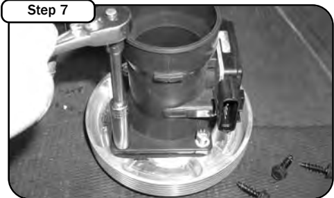
Step 7 Mount the Maf sensor to the billet adapter using the four supplied M6 screws and washers.
