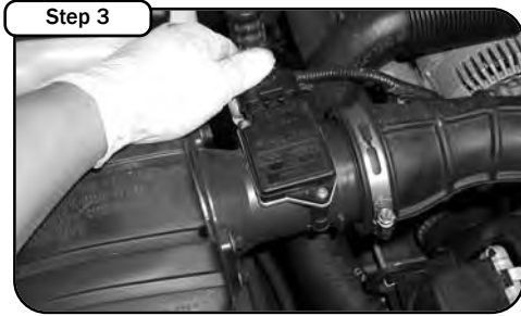
Step 3 Disconnect negative post from battery terminal. Loosen the hose clamp on the intake duct. Disconnect the MAF sensor by pushing down on the clip and pulling out.
