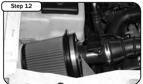
Step 12 Make sure all hoses and clamps are tight and that all electrical components are secure. Re-check after a few hours of operation. Place the included CARB EO Sticker on or near the intake system on a smooth, clean surface. E.O. identification label is required in passing the Smog Check inspection.
