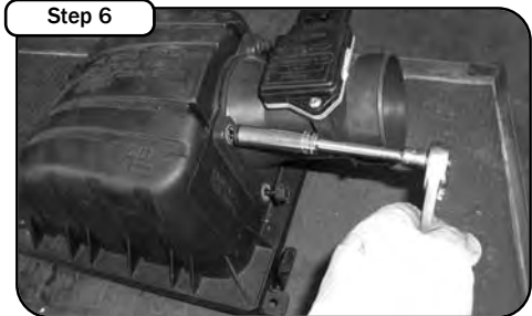
Step 6 Remove MAF sensor from the upper portion of the airbox by removing the four 10mm screws.
