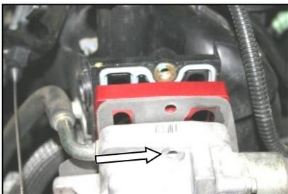
7. Install the top bolt (#2) and washer (#3) first, run it in a few threads with your fingers, leave it loose, and then align the two bottom holes and install the bolts and washers. Use caution not to cross thread the bolts. **Do Not Over Tighten The Bolts!**
