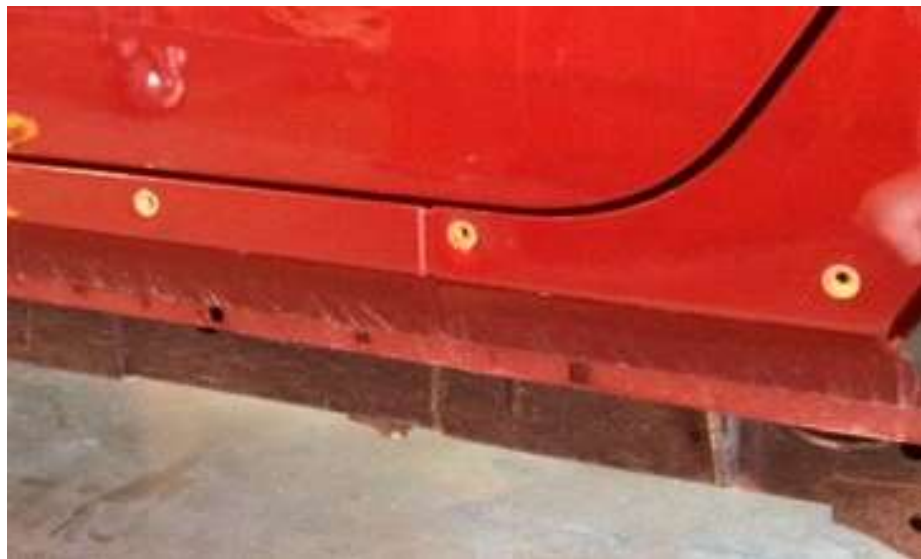
(Nutserts that have been installed correctly)
