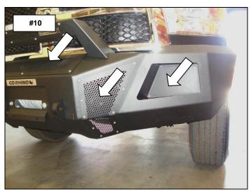
If your state law requires a front license plate, attach the license plate bracket to the holes in the face of the bumper shell, using the supplied 3/8" bolts, washers and nuts, and the license plate to the (2) obround holes in the license plate bracket using the supplied ½" bolts and nuts. (Photo 11).
