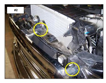
**Step-3** Remove the (2) plastic push in connectors securing the radiator shield to the radiator support using the tip of a screw driver and the bolts (1) per side securing the top of the intercooler to the radiator support using a 13mm socket and ratchet, (Photo 3).
