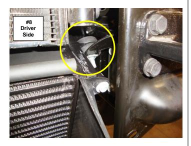
**Step-6** If equipped remove the nuts and bolts (2) per side securing the under rider brackets to the frame using a 24mm wrench, socket and ratchet, (Photo 9).
