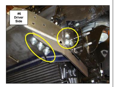
**Step-7** With assistance lift the bumper shell up to the vehicle, align the holes in the bumper shell brackets with the weld nuts on the mounting plate/winch tray and secure the bumper shell to each side of the mounting plate/winch tray using (3) ½" x 1 1/2" hex bolts, (3) ½" lock washers and (3) ½" flat washers, (Photo 7 & 8). Leave the bolts loose for final adjustment.
