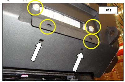
If installing a winch, attach the license plate directly to the (2) obround holes in the lower face of the bumper shell using the supplied 1/4" bolts and nuts, (Photo 14). Remember to check and retighten all factory and supplied nuts and bolts periodically.
