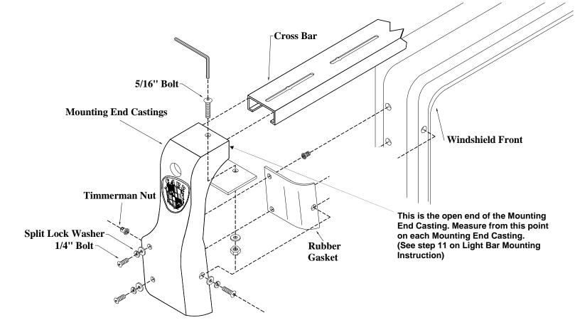
**MATERIALS NEEDED:** Drill motor, 5/16" drill bit, hammer, center punch, <sup>1</sup>/<sub>2</sub>" drill bit, hacksaw.
