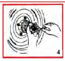
Re-install cover assembly with its gasket. Tighten cover screws or hex bolts to 3.0-4.0 N~m (26-35 in. lbs) using torx wrench "T15".
