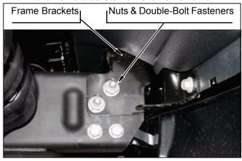
e. Remove four bolts, two nuts and two tow hooks from frame horns.
