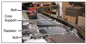
g. Lower intercooler and radiator and install on core support with two bolts.
