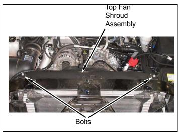
d. Install top fan shroud on bottom fan shroud with four pop-ups. Check fan to shroud clearance. Ensure gap is the same all around shroud.
