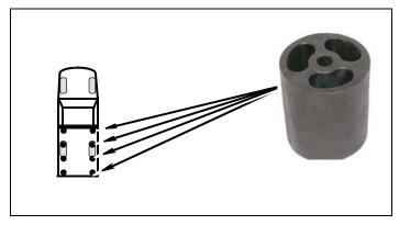
c. Install kit lift blocks on frame and bed with four kit bolts (12mm-1.75 x 100mm) and four kit washers (7/16" USS). Do not tighten.
