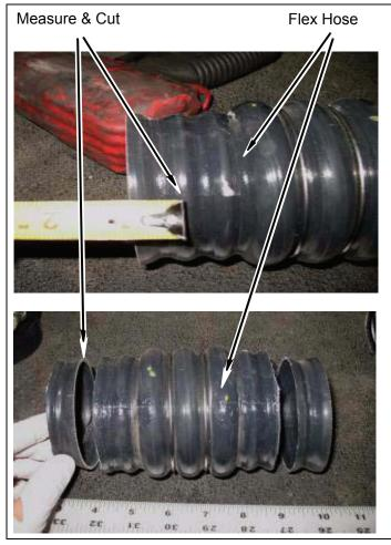
d. Place O.E. Flex Hose onto Upper / Lower intercooler pipe. Install two kit clamps onto intercooler pipe and Flex Hose, do not tigthen kit clamps at this time.
