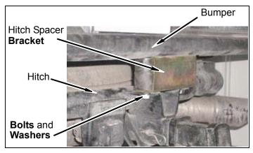
r. Adjust bumper to bed clearance using measurements taken earlier and tighten hitch bolts first then remaining bolts and nuts to 55 lbft. s. Plug license plate light harness in at crossmember connector.
