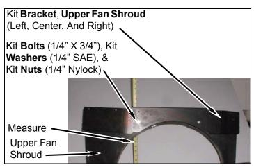
f. Clamp two scrap pieces of metal (or rulers) to fan shroud as shown. Position upper fan shroud on metal scrap and under kit **bracket**, **upper fan shroud** (center).
