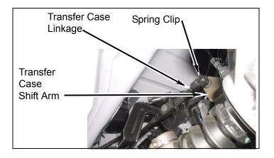
b. Scribe a line along transfer case linkage as shown. Cut transfer case linkage into two pieces through the scribed line and deburr.
