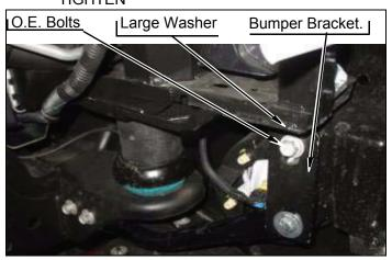
g. Install two bumper supports onto kit brackets with two kit bolts (7/16"-14 x 1-1/2"), four kit washers (7/16" SAE), two kit nuts (7/16"-14 Stover) with four O.E. bolts to body mount. DO NOT TIGHTEN.
