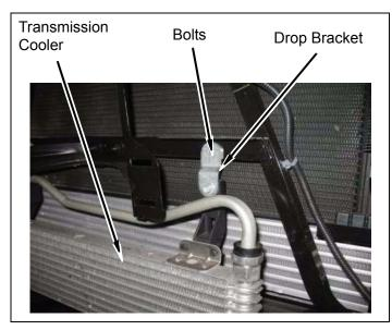
b. Install two *kit* **Spacers** in between lower transmission cooler bracket and core support using *kit* **(3/8 x 2 1/2") hardware**.
