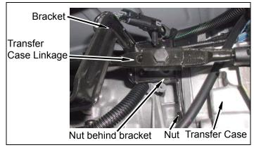
c. Remove two clips and transfer case linkage from transfer case and pivot.
