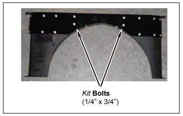
e. Measure kit **bracket**, **upper fan shroud** (center) from table top as shown. Ensure bracket is level.
