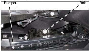
**f.** Install two *kit* **brackets** (bumper, front, support) onto bumper with two *kit* **large washers** between bumper and kit bracket. DO NOT TIGHTEN
