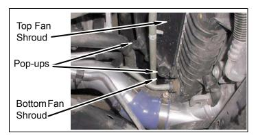
e. Mark & Drill two holes in upper fan shroud bracket using computer module as a templete. Install computer module on upper fan shroud with two pop-up clips.
