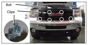
c. Install cover on core support with seven push pins.
