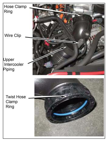
b. Remove Lower intercooler pipe and hose from vehicle by twisting ring clip.
