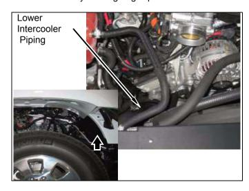
c. Remove clip and harness from engine mounted bracket.
