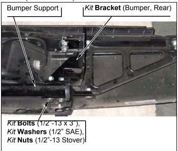
**m.** Install bumper support and two *kit* **brackets** (bumper, rear) onto bumper with two O.E. carriage bolts and six nuts. DO NOT TIGHTEN.
