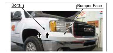
b. Position grill on core support and install six clips and four bolts in core support and front fenders.
