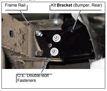
**h.** Mark eight holes through two *kit* **brackets** (bumper, rear) onto bumper support.
