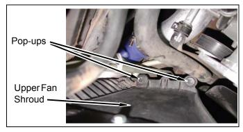
d. Remove computer wiring harness from harness push clip and lower fan shroud.
