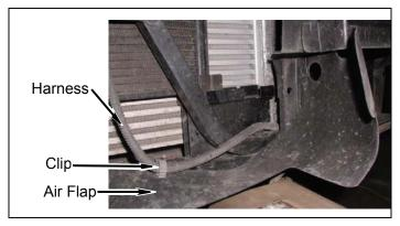
d. Remove two clips, three push pins, and air flap from core support.
