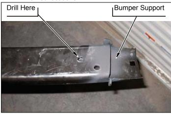
I. Install bumper support onto two *kit* **brackets** (bumper, rear) with four *kit* **bolts** (1/2"-13 x 3"), eight *kit* **washers** (1/2" SAE) and four *kit* **nuts** (1/2"-13 Stover). DO NOT TIGHTEN.
