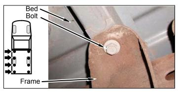
b. Remove four bed bolts from frame passenger side.
