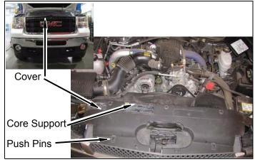
b. Remove four bolts, six clips, and grille from core support. Some GMC models may have extra clips.
