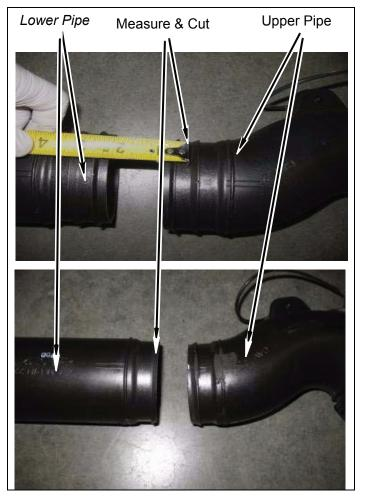
c. \*Measure and Cut\* O.E. Flex Hose. \*Measure and Mark\* 3/4" from EACH end of the Flex Hose. \*Carefully cut Flex Hose. Be sure to clean ALL particles from Flex Hose.
