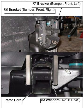
c. Install frame bracket onto kit brackets (bumper, front) with two kit sleeves (.75" OD x .532" ID x 3.35" L), four kit bolts (1/2"-13 x 5-1/2"), eight kit washers (1/2" SAE) and four kit nuts (1/2"-13 Stover). DO NOT TIGHTEN.
