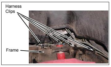
b. If possible, install two brake lines in two sets of clips. If brake lines will not fit back into position, wrap lines with two kit **zip ties** individually, and then secure the lines together with one kit **zip tie** as a bundle.
