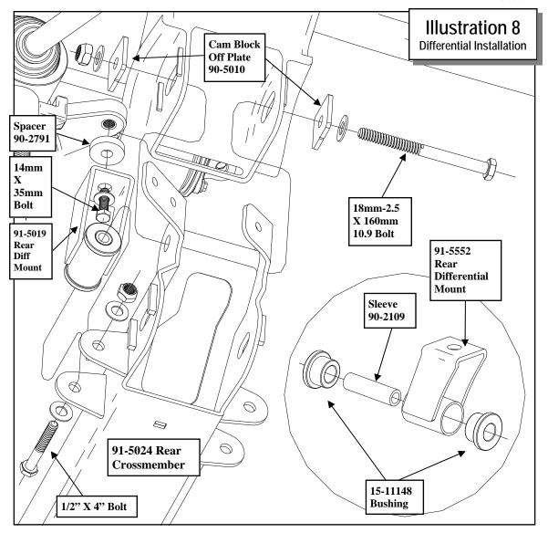
NOTE: Carefully guide the rear of the passenger side differential mount (90-5246) into the mounting tabs on the rear crossmember during installation.
