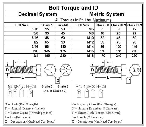
Use this only as a guide for hardware without a called out torque specification in the instruction manual.
