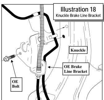
ing hole in the frame. Secure using the previously removed **OE** bolt. See ILLUSTRA-TION 17.
