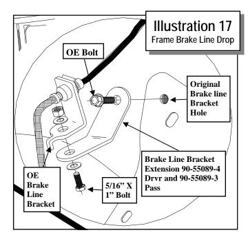
pull down the factory metal lines to provide an adequate amount of slack. DO NOT kink the lines.
