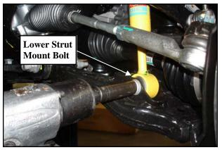
8. Remove the ABS bracket from the A-arm.
