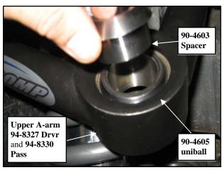
21.Using a floor jack, raise the lower A-arm and knuckle and secure the upper ball joint mount to the knuckle using the supplied 9/16" X
