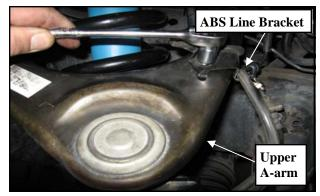
Loosen, and remove the upper strut nut on the strut tower (4) on each side of the vehicle that holds the strut assembly to the strut tower.
