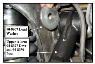
20.Insert spacer (**90-4603 top** and **90-4604 bottom**) into the uniball ) on the Pro Comp upper A-arm.
