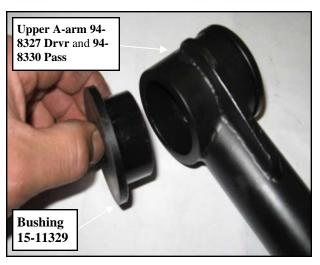
15.Insert the sleeve (**90-8331**) into the upper A-arm bushings.
