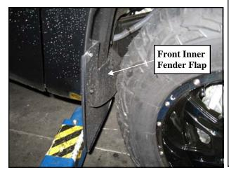
ing hole will also have to be redrilled in it's new position.
