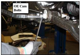
6. Unbolt the sway bar end links from the lower A-arm. Save the hard-ware for reuse.
