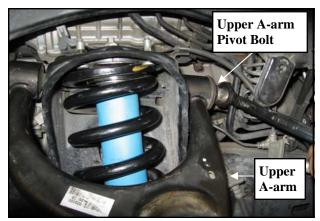
12.Remove the upper A-arm from the vehicle. Save the **OE** hardware for reinstallation.
