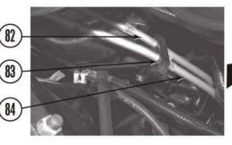
f. Remove nut (85), two wire loom brackets (86), bolt (87), clamp (88), and two oil cooler lines (82 and 84) from oil pan (89).
