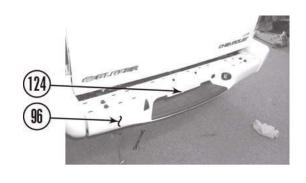
b. Trim inside of rear bumper (96) in two places as shown. Test fit bumper to ensure that enough material has been removed.
