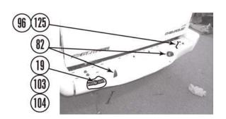
e. Install two *kit* rear bumper brackets (125) on frame (19) with two double stud fasteners (100), four nuts with captive washers (99), four *kit* 7/16" x 1 1/2" bolts (129), eight *kit* 7/16" USS washers (127), and four *kit* 7/16" nylock nuts (128). Do not tighten.
