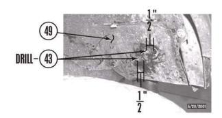
d. Install differential actuator (47) and bracket (48) on wheel well (49) with two bolts with captive washers (46).
