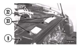
c. Install upper fan shroud (32) on lower fan shroud (34) with four *kit* 3/8" USS washers (136), four *kit* 3/8" x 3 1/2" bolts (137), four *kit* tubes (138), four *kit* 3/8" USS washers (136), and four *kit* 3/8" nylock nuts (139).
