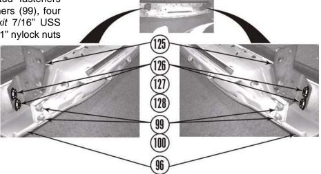
d. Loosely position two kit rear bumper brackets (125) and rear bumper (96) on frame (19) and install two license plate lights (82), three clamps (103) and harness (104) on rear bumper.
